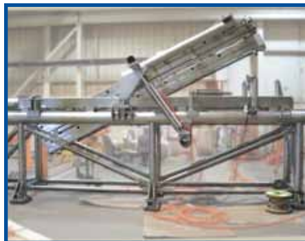
Center Pivot Transfer System (CE)
