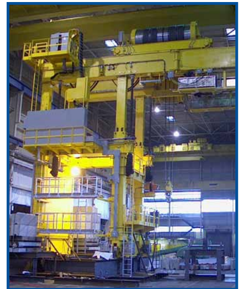
110/45 ton X-SAM® cask handling crane with mechanized telescoping legs and extendable girders
