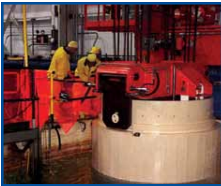
130 ton X-SAM® cask handling gantry crane with multi-cask lifting device integrated into load block
